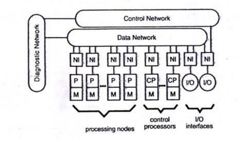
Input and output were provided through high bandwidth I/O interfaces to graphics devices, mass secondary storage such as data vault, and high performance networks. Additional low-speed I/O was provided by Ethernet connections to the control processors. The largest configuration was occupy the space of 30m x 30m and designed for a peak performance of 1 Tflops.
