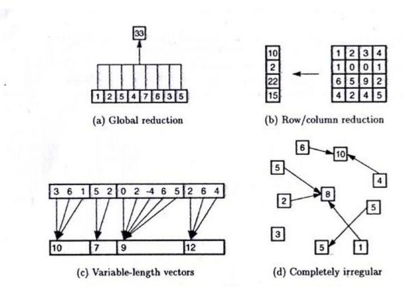
**<u>Permutation</u>**: Data parallel computing relies on permutation for fast exchange of data among processing nodes. The following diagram shows four cases of permutations performed on CM-5. These permutation operations are often needed in matrix transpose , reversing vector, shifting a multidimensional grid, and FFT butterfly operations.
