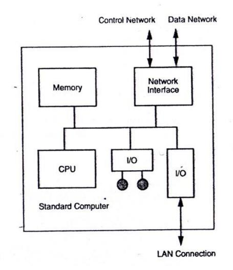
Each control processor ran CMOST, a UNIX based OS with extensions for managing the parallel processing resources of the CM-5. Some control processors managed computational resources in user partitions. Others were used to manage I/O resources. Control processors specialized in managerial functions rather than computational functions.
