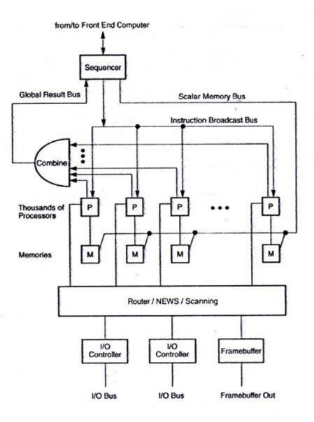
Global combining allowed the front end to obtain sum, largest value, logical OR etc.. of values, one from each processor. The scalar bus allowed the front end to read or to write one 32-bit value at a time from or to the memories attached to the data processors.
