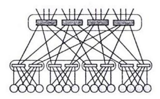
To implement the partitions, one could allocate different subtrees to handle different partitions. The size of the subtrees varied with different partition demands. The I/O channels were assigned to another subtree, which was not devoted to any user partition. The I/O subtree was accessed as shared system resource. All leaf nodes had unique physical addresses.
