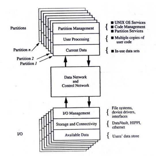
Partitioning of resources was managed by a system executive. The control processor assigned to each partition behaved like a partition manager. Each user process executed on a single partition but could exchange data with processes on other partitions. Since all partitions utilized UNIX time-sharing and security features, each allowed multiple users to access the partition.
